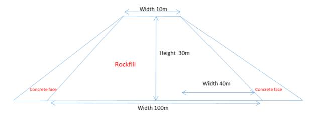
For example, considering the dam as a structure as per the above, the user can calculate the relative amounts of materials required. For the rockfill, the cross-sectional area can be estimated as:
