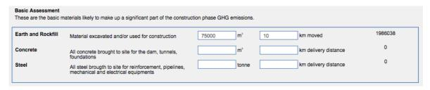
Similarly, this can be done for concrete and steel. Users should consider the approximate amounts of material in the dam, tunnels, powerhouse, and other assets, following a similar approach to the above if information does not exist on the amounts of those materials in the project.
